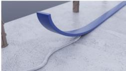
Alternatively, the swelling tape is fixed by nailing at approximately 150mm centres.
