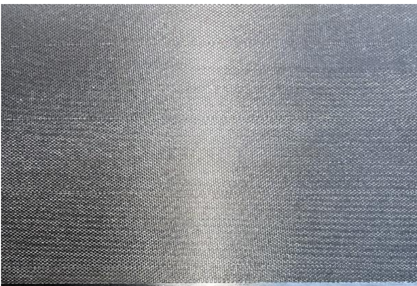
Picture 2 - Dural CFP plate with protective film removed. Note the textured finish.
